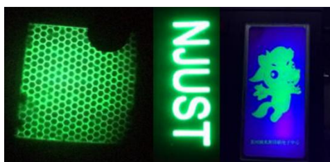
Fig. 1 Various robust photo/electro-luminescence patterns by directly ink-jet printing the CsPbBr 3 QDs.
